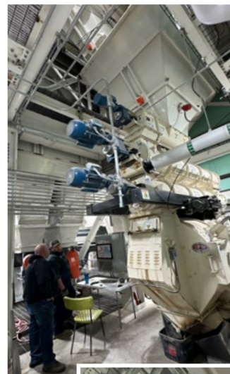
Conditioner & pelletizer, fed by a conveyor belt from the mixer.
