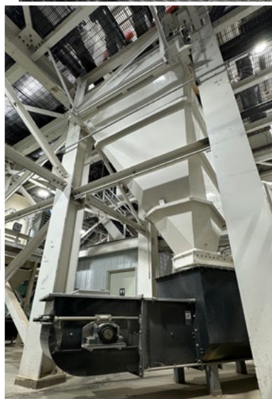
Ingredients are each weighed on the scale and sent out to the (existing) mixer.
